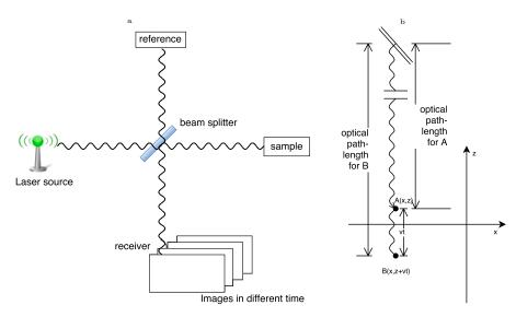
Fig. 1. a) Illustration of the imaging setup. b) A particle moves from A to B covering a distance of vt. When the particle is at B, the light travels an additional distance of 2vt inside a medium with refrative index  $\bar{n}$ , so the effective path-length of the sample arm increases by  $2\bar{n}vt$ .
