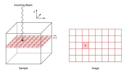
Fig. 2. One "slice" in the sample, and its division into small regions corresponding to the pixels of the image.
