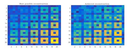
FIG. 9. Reconstruction of the metabolic map presented in Figure 4. The left image corresponds to using directly formula (26) on the isolated  $A_m$  signal. The right-hand image corresponds to using our reconstruction method on the total signal. Once the images are normalized, the committed error with respect to the original metabolic map is 0.011 and 0.017, respectively.
