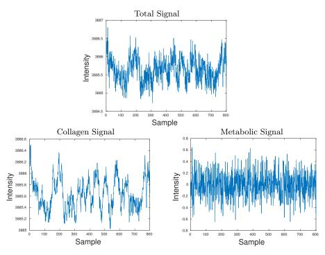
FIG. 3. On top we can see the total signal measured at a fixed pixel. If decomposed into the one corresponding to the collagen structures and metabolic signal, we obtain the bottom images, left-and right-hand side, respectively.
