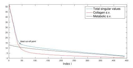
FIG. 6. Singular values for the signals. The circle represents the optimal starting index j at which we should consider the singular space-vectors of the total signal to contain mostly information on the singular space-vectors of the metabolic activity. The first singular value of the total signal and the collagen signal is outside the plot, with an approximate value of  $2.3 \times 10^6$ .
