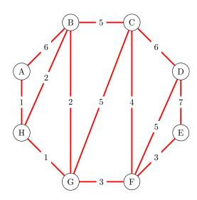
Apply the greedy algorithm to find the minimum spanning tree and it's cost. Is it unique? Write the sequence in which the edges are added to the minimum spanning tree.
