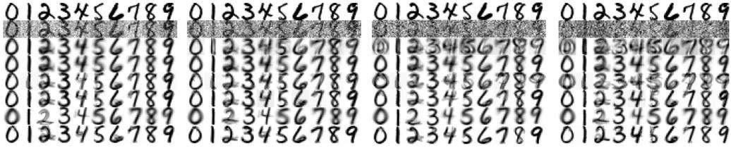
Figure 6: Digit images corrupted by additive Gaussian noise (from left to right,  $\sigma^2 = 0.25, 0.45, 0.65, 0.85$ ). The different rows respectively represent, from top to bottom: the original digits; the corrupted digits; denoising with [10] ; with [10]+[1] ; with [20] ; with [20]+[1] ; with [4]; with our Karcher mean interpolation based method. See Table 2 for quantified results
