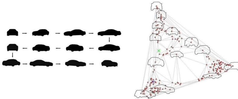
Figure 8: a) 12 shapes for one of the 17 cars used in the dataset. b) Reduced space of the car data set and its Delaunay triangulation.
